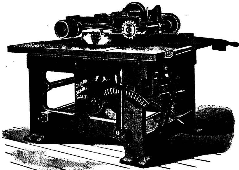
...Our No. 24 Variable Self-feed Rip Saw. A simple, substantial saw, designed for heavy work in Planing Mills, Furniture and Sash and Door Factories.
