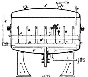
the vessels containing the substance to be sterilized, and movable presser-bar mechanism for operating the closing wires of the vessels, substantially as described and illustrated.
