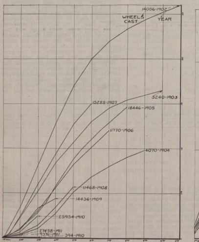
Fig. 9.—Failures Caused by Manufacturers' Defects on Wheels Cast in Successive Years for 80,000 lbs. Capacity Cars for C.P.R.
