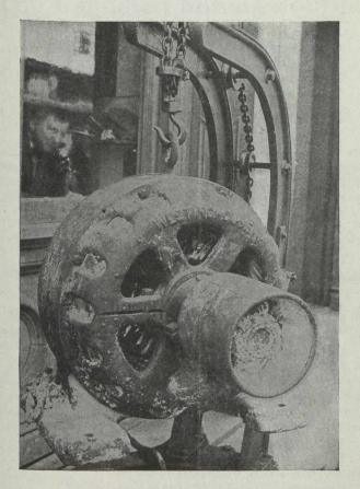
Note the incrustation of salt in the pulley, around the terminals, and especially on the rotor fans and stator windings. Needless to say, a good deal of this salt was shaken off during transit, but in view of the water absorbing quantities of rock salt, there is sufficient remaining to indicate the conditions under which the motor was used.
