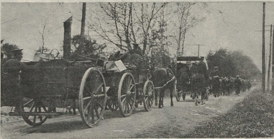
The "Cooker" or Field Kitchen makes the life of the soldier much easier—it trails along at the end of the column, cooking as it goes. When the column halts, dinner is ready.
