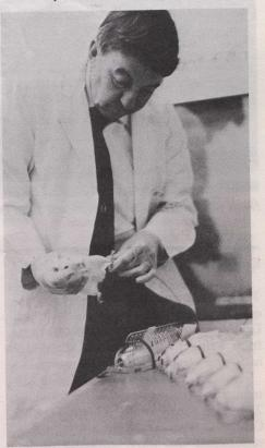
Dr. Olivier Héroux attaches a thermocouple to the body of a rat before it is placed in a restraining cage. This device will monitor the rat's body temperature continuously, enabling the researcher to record the information without disturbing the animal.
