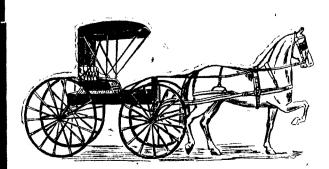
224 C-PIANO BOX BUGGY—Wheels, Sarven. I-in. tire; Axle, 15|16-in.; Painting, body black, gear, dark green; Trimmings, leather, spring back and cushions with carpets in bottom of box, nickle rail and caps on hubs. With shafts only .......65.00
