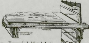
built with steel studding—Expanded Metal Lath and Solid Plaster, on both sides, are the only reliable fireproof partitions.
