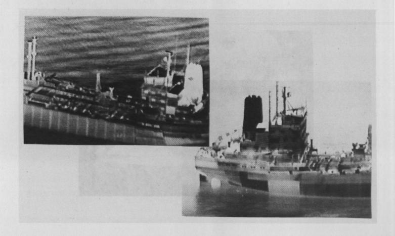
Figure 10. FLIR images of freighters. Notice the hot stack in the left image and the ability to "see through" the hulls because of differences in surface temperature resulting from contents of the holds. (Courtesy of David Dorschner, Aviation Resource Management.)
