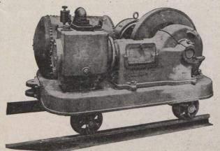
The construction of the air compressor is very substantial. The bearings are all adjustable and removable. The cylinder is lubricated by a light feed air cylinder lubricator and the crank shaft and crosshead by the splash system. An unloading device on the air inlet valves saves energy when the demand for air is less than the output of the machine.
