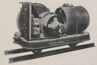
The motor is of the damp proof type and will operate successfully in the wettest portions of the mine. It is supplied for either alternating or direct current.
