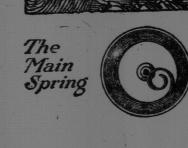
THE mainspring is the power of a watch. It is a piece of specially hardened and tempered steel, about twenty inches long, coiled in a barrel between the upper and lower plates of the movement. It is subjected to varying conditions of service in temperature and tension. The variation in thickness of two one-thousandths of an inch, or lack of uniformity in hardening, and tempering will decide the time-keeping quality of your watch.
