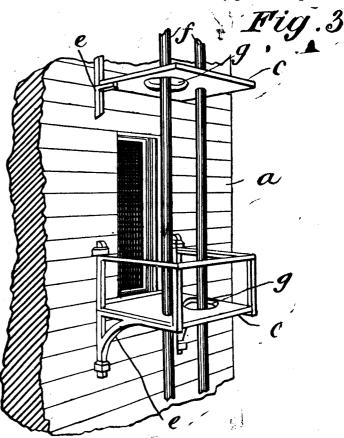
floors or staging from the root to the ground; g g are circular openings which alternate from one side to the other at each succeeding landing. The landing to be placed before a window at every story.
