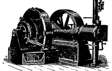
THE above cut represents a ROBB-ARMSTRONG Engine direct connected with dynamo. Simple, Tandem, or Cross Compound Engines may be used combined with any standard type of Dynamo.
