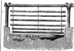
companying engraving is well adapted for the pur-The one at the top is made from poles of pose the desired length woven together with strong wire which, in turn, is secured to the overhanging pole As the water rises the poles float upon its surface and do not in the least impede its onward progress. | and not pedigrees.
