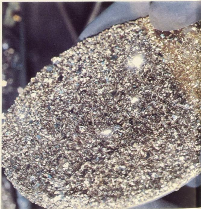
In studying high temperature thermal conductivity, physicists require metal specimens of consummate purity. These crystals of strontium were grown in an insulated container under an atmosphere of dry helium gas.
