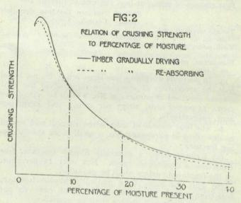
grees of dryness, as shown by fig. 2, seems to show that the greatest strength is reached not when the wood is absolutely dry, but with some 3 per cent. or 4 per cent. of moisture. It is somewhat difficult to ascertain this with perfect accuracy as absolutely dry wood re-absorbs moisture so rapidly from the air; it is how ever not a point of practical importance as such dryness condition as 3 per cent. is never found in actual practice.
