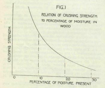
eral specimens cut from the same stick of timber, the specimens being of different degrees of dryness. Plotting the strengths to a base of moisture percentage gave a curve of the form shown in fig. 1.
