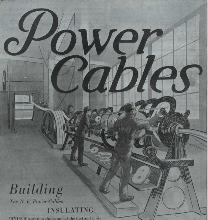
THIS illustration shows one of the first and most I important steps in the manufacture of N. E. Power Cables—the covering of the conductor with paper insulation.
