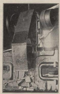
Fig. 2.—Gear Protection on Punch Press.
