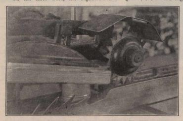
Fig. 3.—Protection to Star Feeder on Rip Saw.
