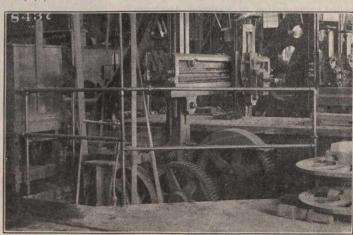
Fig. 4.—Protection to Planer Gearing.
