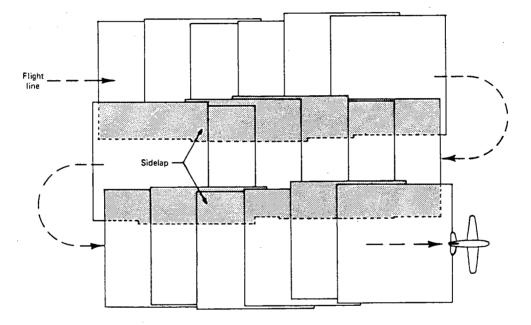
Figure 3. The use of sidelap between adjacent flight lines to obtain contiguous coverage of a project area. (Source: Lillesand and Kiefer, op. cit., p. 80.)
