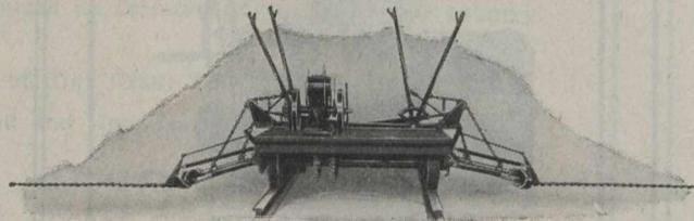
Cutter Bars easily raised, lowered and tilted up or down while cutting, to follow grade surface.
