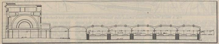
Fig. 4. Cross Section through Union Station and Passenger Subway under Tracks, showing Interior Arrangement.
