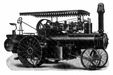
There is not another tractor like this under the sun except another Big Forty. It's different in its quick-steaming, well-made boiler; its four (double tandem compound) cylinders; its evenly balanced, strong crank shaft running in four journals; and the distinctive style of its rear-mounted traction gearing of steel and semi-steel.
