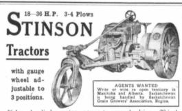
36 h.p., 4 cylinder motor—power to properly drive a 28-inch separator—kerosene burning at all loads—3000 lbs. draw-bar at 3 miles per hour—plows 12 to 16 acres in 10 hours, according to number of bottoms-weight 7,130 lbs.-all gears enclosed, running in oil—and it can be bought at the same price the American farmer pays. Get catalogues and full information.
