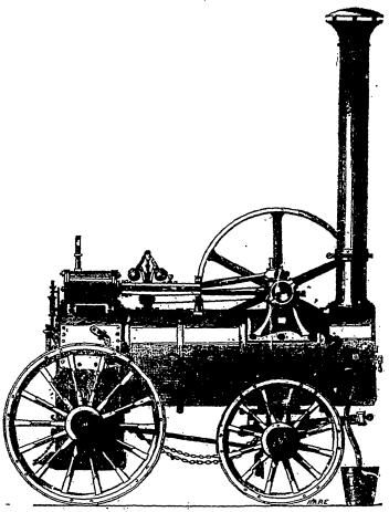
dages necessary to render them complete. It has a crank shaft which is much superior to the old over nick crank, and admits of the fly wheel being placed on either side of the boiler, or a pulley being placed on the opposite side to the fly-wheel of dimensions suitable for working any additional machinery.
