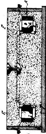
34555 Bouton's Mode of Making Sectional Chills.
