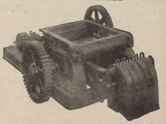
Capacity Single Roll Crusher 50 to 70 tons an hour.
