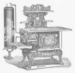
This cut illustrates a Jewel Range connected with Galvanized Water Boiler. The range is fitted with Waterfront which is tapped for one-inch pipe and connections to boiler should be the same size. In making connections sharp angles should be avoided as much as possible. Do not in any case make a fire in range before the boiler is filled with water.
