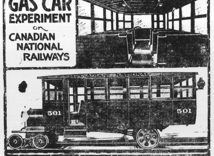
This gasoline-driven equipment is being experimented with by Canadian National Rallways on its line out of Brockville to Westport, Ontario. It makes four round trips, or a total of 855 miles per day. It is required to run 45 miles in 1 hour and 45 minutes, including all stops. This car is handling a large number of passengers daily.
