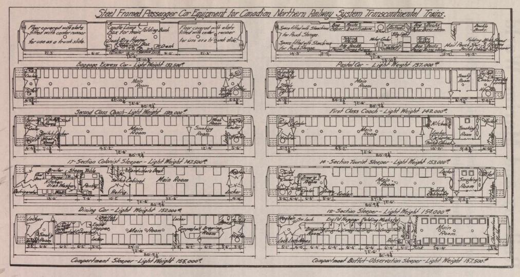
Experience gained from service of a large number of colonist sleeping cars, caused the railway company to provide ample facilities for washing and cooking which are absolutely essential for this type of equipment. The usual square deck and finish throughout was employed, the interior being of natural birch. Ample ventilation and large water supply is necessary also for a large smoking room.
