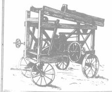
THE Noiseless Well Drilling Machine is the term usually applied to The Standard when compared to other makes, with their incessant rattle and clang. They are compactly constructed and their mechanism is built of iron and steel—not wood.
