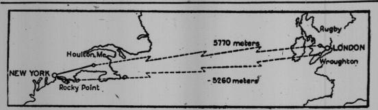
Air paths used in the first successful two-way radio telephone tests between New York and London are shown by this chart. For transmission from New York, wire links from Manhattan to Rocky Point and from Wroughton to London were used. The Britons did their chatting over wires from London to Rugby, thence radio to Houlton, Me., and on by wire to New York,
