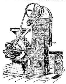
As shown, are now fitted with a Shaking Screen to take out all Straws, Stones, Nails, Cyl. Teeth, etc.
