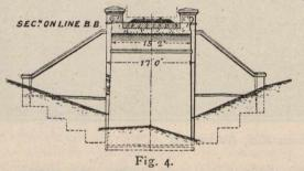
thick at the crown, and 5'-o" at the springings. It has a rise of 28'-o", and is 15'-6" in width. The spandril arches are 13'-o" span, with a rise of 3'-o", and 12" thick at the crown. A temperature range of  $48^{\circ}$  Fahr., was allowed for in the design. The excellence of the material at hand: in the shape of stone, sand, and abundance of water, led to
