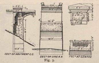
the questions of loading, a rather more irregular curve than that adopted would have been the more correct. The calculations were worked out in accordance with Professor Cain's elastic theory. A live load of 1.875 tons per lineal foot of bridge was taken, this being nearly 20 per cent. in excess of the heaviest engine load in use.
