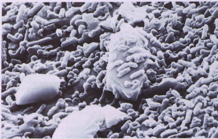
Bacteria colony ( Thiobacillus ferrooxidans ) of leaching microbes (electron micrography X 7500). These bacteria digest pyrite or iron sulfide and release the precious metals.
