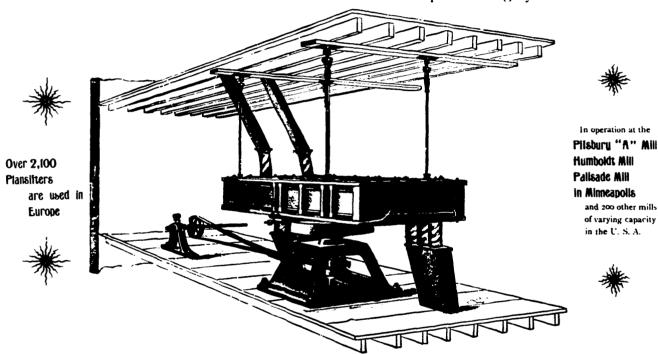
One Single Plansifter will do the entire Scalping, Grading and Bolting of a mill of 40 to 60 barrels capacity
