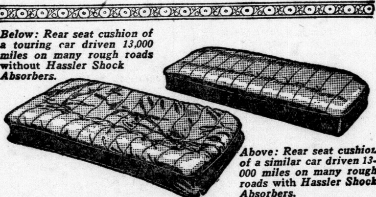
Below: Rear seat cushion of a touring car driven 13,000 miles on many rough roads without Hassler Shock Absorbers.
