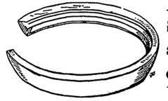
Shows Bezel of Keystone Case made from a solid piece of sheet silver by swedging dies.
