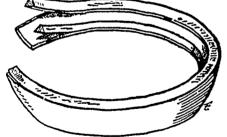
Shows Bezel as commonly made with three pieces of silver soldered together.
