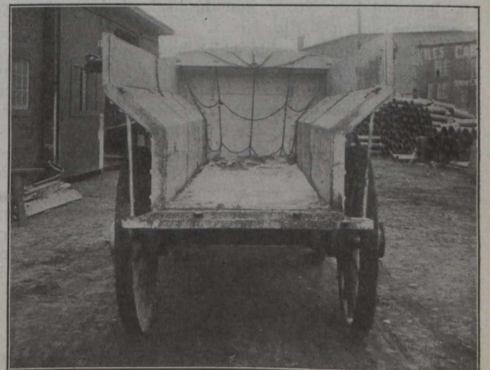
Fig. No. 2.—Tail-board Down; Unloading Device in Place Ready for Another Load
