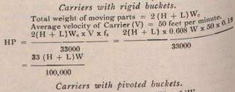
Total weight of moving parts =  $2(H + L)W_c$ Average velocity of Carrier ( $\mathbf{V}$ ) = 50 feet per minute.  $2(H + L)W_c \ge V \ge f_s = 2(H + L) \ge 0.756 W \ge 50 \ge 0.35$
