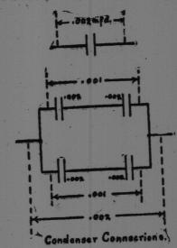
In receiving circuits, fixed or variable condensers are used in series with the antenna circuit in order to reduce the wave-length for receiving purposes. The wave-length may be increased for receiving longer wave-lengths by either inserting a loading coil in the antenna circuit or by shunting (placing in parallel) the primary coil of the coupler with a variable condenser.
