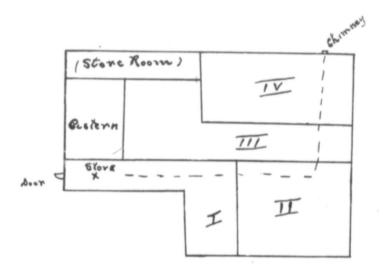
A "Tribune" stove was placed near the cellar door, which communicated with the outside; and through this door the fresh air from the outside had access. The air in its natural course, by means of the openings around the stovepipe, passed from room to room; and finally in the fourth room passed out by means of a similar opening in the chimney,—the same chimney into which the regular pipe entered. This chimney has in addition, a pipe entering it from the stove used in the living room above.
