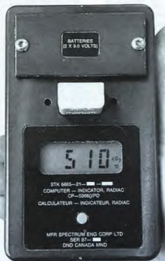
With the locket in place, the reader provides accurate dose readouts on its LCD display.
