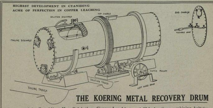
Constructed for Cyaniding, Hypolixiviation, Copper Leaching, and Chlorination; combining Agitator Filter, and Washer. Highest extraction in shortest period of time: saving labor, power, and chemicals.
