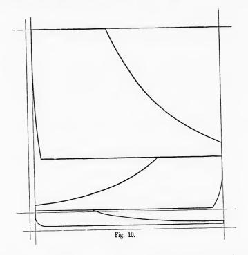
the theoretical diagrams, unless an allowance is made in the cylinder ratios to compensate for the progressive loss occasioned by condensation in the cylinders.
