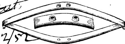
All now made with Armstrong's patent re-enforced holes (see centre of cut). These being punched without loss of stock leave the spring fully stronger there than at any other part of the plates, and being recessed into the bearing block in attaching, take away all wear or strain from the bolts, doing away with former objections to bolting, and making a very secure fastening.
