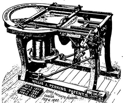
The only Horizontal Saw Machine on which a thick -lab can be cut from the bolt. SECOND CUT ALWAYS A SHINGLE. Knots, rots, hearts, bolt squared rift-ways, and all irregularities cut off at one clip. This improvement will pay price of the whole machine every season by increase of quality and quantity cut.
