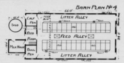
quirements. Walls are sheeted with resawn lumber and siding up to the top of stable joists, with siding above up to the caves. The stable is lined with shiplap. Specifications call for the loft floor being tongued and grooved flooring, but paper and another ply of wood on the floor would eliminate dust falling into the stable below. To reduce the cost of this extra ply of flooring, two ply of common lumber and paper can be used.
