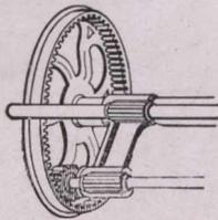
Space prevents reference to the many splendid features of the Frost & Wood Mower, but the "Internal driving gear" as shown here must be mentioned. The driving gears are meshed on the inside of the main drive—travel in same direction—no tendency to fly apart, or to snap cogs—no loosening or rattling of parts and connections, and the knives begin to cut at the first step of the horses. This means quicker work and longer life to the machine.
