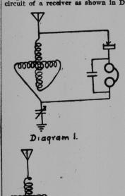
ance to the currents of radio frequency than a tuning coil having the same amount of inductance. For use on the amateur wave length of 200 meters, the variometer may have an inner coil three and one-half inches in diameter, wound with 20 turns of No. 24 S.S.C. wire and an outer coil four inches in diameter, wound with 15 turns
