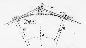
If the front tangent has not been located, in beginning the circular curve proceed as follows. Set up transit at offset distance inside the tangent, or at the P. C.; backsight to a point similarly offset; then run the curve as usual. At the P. T. the operation will have to be reversed. If, on the contrary, the front tangent has been fixed, T and not T, must be measured from the vertex to locate a point from which to lay off F from the P. C.,  $T^{i}=$
